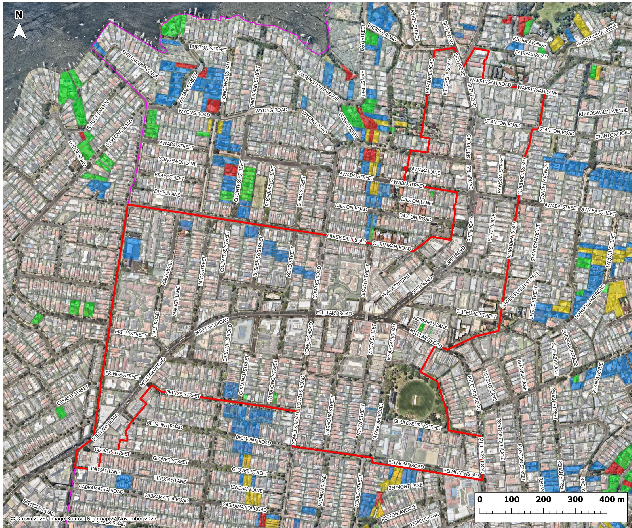
Figure 2-2 Flood emergency response classifications during 1% AEP event
